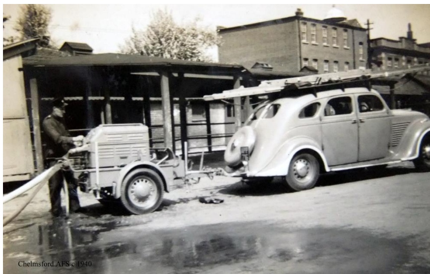
Chelmsford's AFS powerful American towing car with its Beresford-Stork light trailer pump. (EFM Archive
