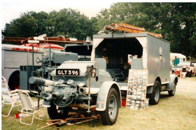
A preserved Austin ATV and trailer pump similar to EFM's GXH 472. These pictures show the vehicle in its original form. (EFM Archive)
