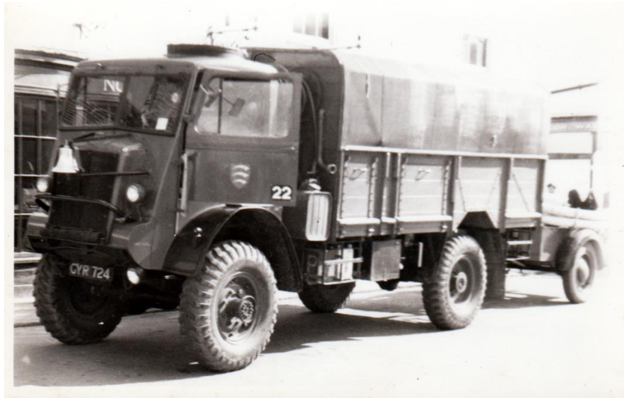
An ex-Army Bedford QL lorry operating as a fire engine with a trailer pump from Rayleigh fire station in the early days of Essex County Fire Brigade.(EFM Archive)
