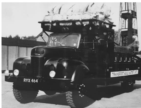
Commer Q4 Superpoise 4x4 Transportable Water Unit, note the three large 'bags' on the roof containing the inflatable rafts. (EFM Archive)
