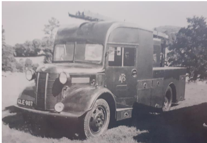
Typical of Ex NFS vehicles issued to the AFS, was this Austin K4 Heavy Pumping Unit (EFM Archives)
