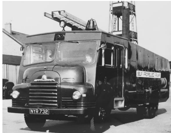
The iconic 'Green Goddess', a 1953 Bedford SLHZ Emergency Self Propelled Pump of the Essex AFS, seen at the Suffolk Road, Seven Kings, Ilford, AFS Depot. (EFM Archives)
