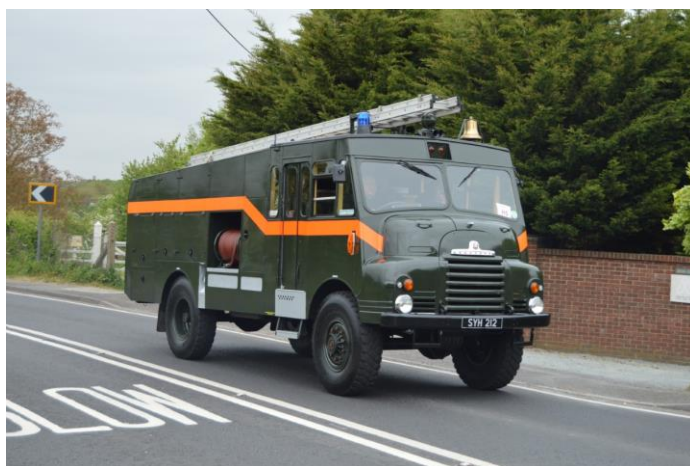
Bedford RLHZ 4x4 Self Propelled Emergency Pump(Photo by kind courtesy of Tony Knell)
