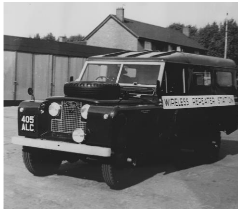
Land Rover Series 2 General Purpose Vehicle, used as a Wireless Repeater Station. (EFM Archives)
