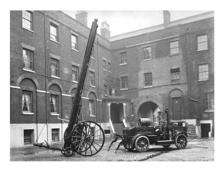
An early Merryweather Motor Escape Van, showing the 'First Aid' hose reel. The water tank is under the driver's seat. (Photo courtesy of the London Fire Brigade).
