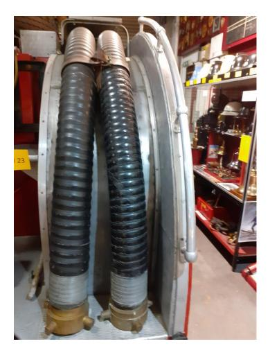
Suction hose, carried on a fire appliance from the 1950s. Modern suction hose differs only slightly from this type of hose.
