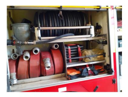
A typical 'hose' locker on a modern fire appliance, showing the hose reel tubing on it's rotating drum, ready for use.
