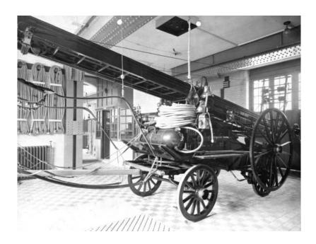
A Horsed Escape Van of the London Fire Brigade from around 1910, showing the 'First Aid Hose' coiled up next to the Coachman's seat. The water was supplied from the large pressurised copper water tank on the foot-board. (Photo courtesy of the London Fire Brigade).
