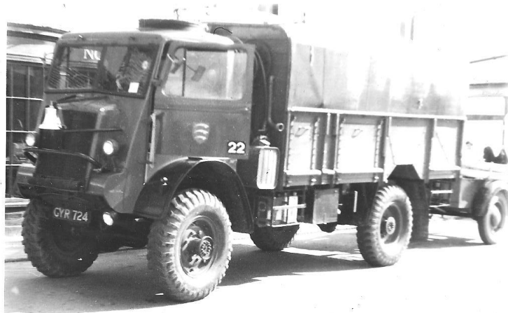
1944 Bedford 'QL' Water Tender based at Station 22 Rayleigh Note the trailer pump 'on tow'
