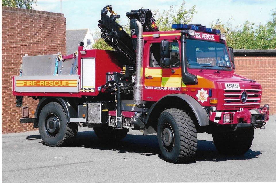
2010 Mercedes Benz 'Unimog' 4x4 Animal Rescue Unit. Seen when based at South Woodham Ferrers, this vehicle is currently based in Chelmsford. (Photo by kind permission of Alan Field)
