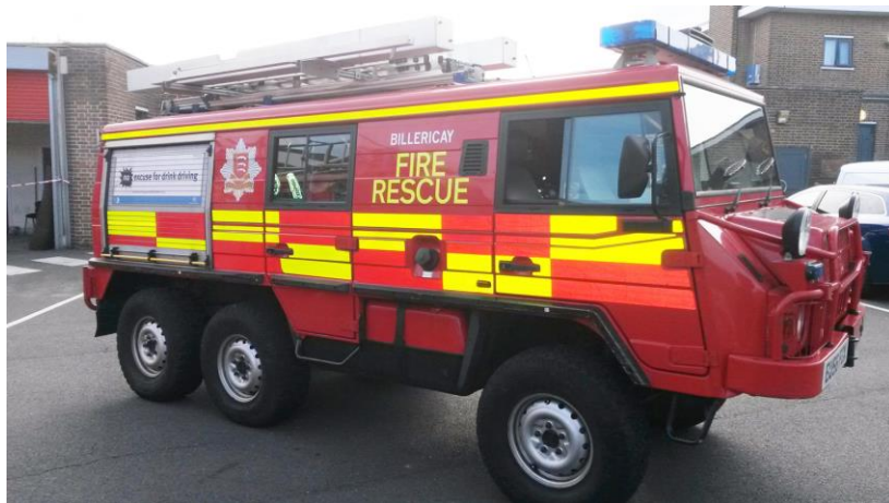
Billericay's 2006 Steyr Puch Pinzgaur/JDC 6x4 Light Water Tender (Photo by M. Beale)
