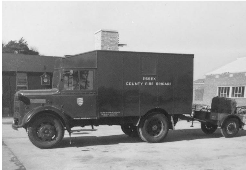
An ATV being used as a Mobile Repair Van (MRV). It was finished in Dark Green and has windows added to the rear bodywork. Inside the vehicle would have been a work-bench and cupboards for tools and spare parts, plus an oxy acetylene welding plant. Note the absence of a bell or ladder gantries. (EFM)
