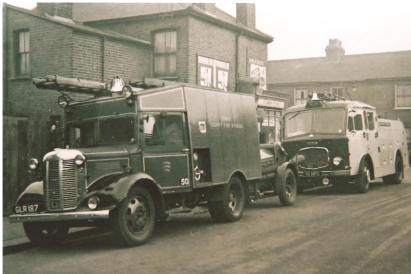
Hatfield Peverel's ATV in attendance at a major fire in 1961. Notice the control panel next to the passenger door, it was part of the Home Office hose reel kit that was fixed on the inside of the vehicle. The hose reel tubing could be pulled out through the small hole just above the control panel. This vehicle also has a lowered ladder arrangement to enable it to fit into its home station. (EFM)
