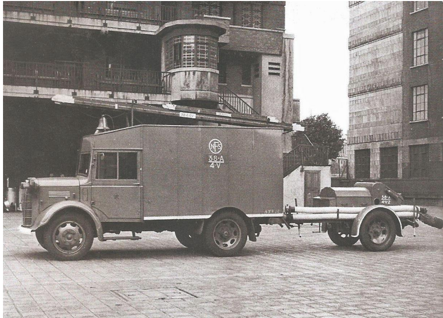
An Austin K2 ATV of National Fire Service No. 38 Fire Force (London) in standard grey finish, It is towing a Dennis No 2 Major Trailer Pump. (Picture courtesy of the London Fire Brigade)
