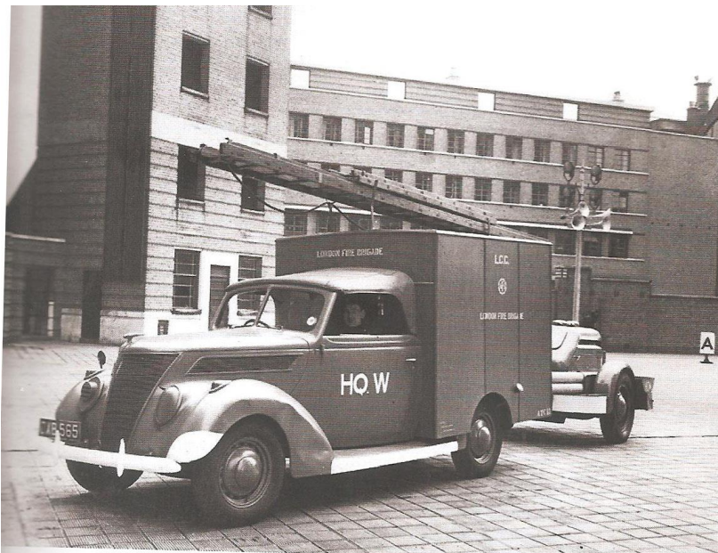
A Ford V8 of the London AFS with the rear part of the car removed and a box body added. (Picture courtesy of the London Fire Brigade)
