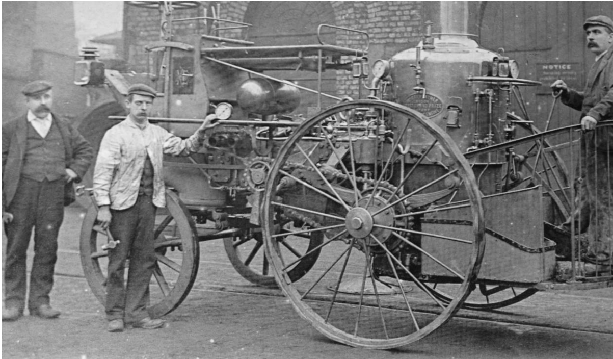
Stand Mason Steamer of Brewery Fire Brigade, capable of throwing a ton of water through a 1 inch nozzle to a height of 80 ft
