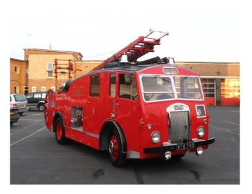
The 1953 Dennis F12 Pump Escape which is part of the Essex Fire Museum's fleet of vintage fire appliances. It has a Rolls Royce 8 cylinder B80 engine, Dennis 1000 gpm (4,500litre) per minute pump and a Bailey's 50ft (15.4 M.) Wheeled Escape ladder.
